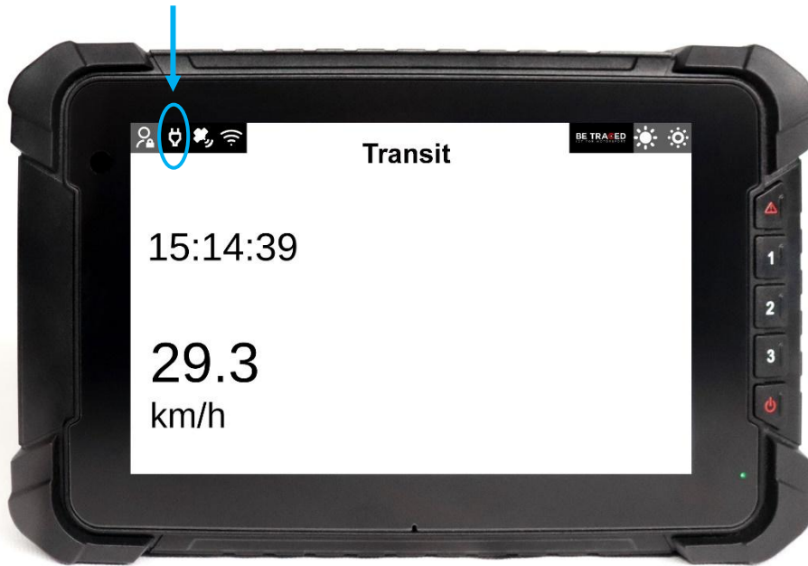
Figure 1 - White power light: device powered correctly
