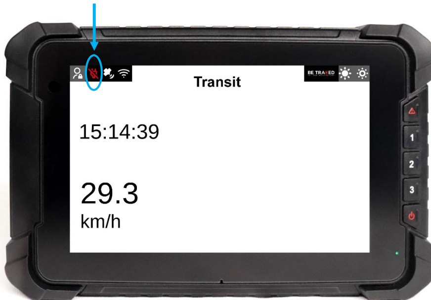
Figure 2 - Red power indicator light: device not powered
